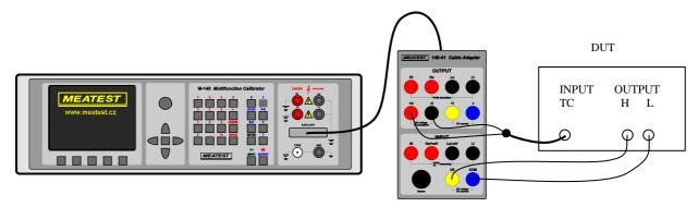
Function setup: Calibrator T TC function
