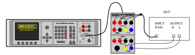
Function setup: Calibrator T RTD function
