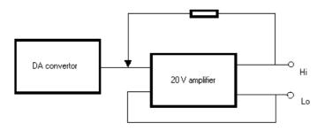
There is a DC reference voltage source integrated within the 22bit measurement converter. Its output is fed to the output stage for 2 and 20 V range. Output voltage present at Hi and Lo terminals is sensed by sensing wires. Feedback eliminates the influence of amplifier's output impedance and of the resistance of wires within the calibrator.
