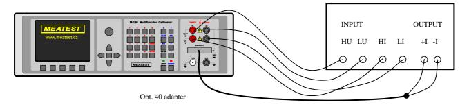
Function setup: Calibrator P function (voltage, current, power factor, frequency)
