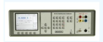
Multifunction calibrator M-142i is calibrator determined mainly as standard of electric voltage and current in calibration laboratories. It can be used for calibration, testing and adjustment of voltmeters, ammeters and multimeters
