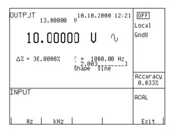
If too large or too small value is entered, the calibrator displays the maximum (minimum) value which is allowed for the selected function.
