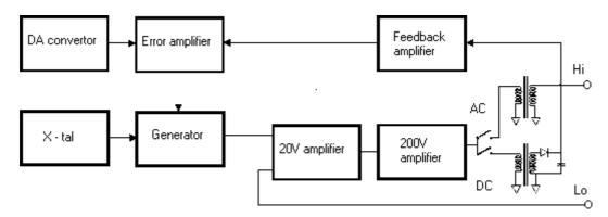
In 1000 V AC mode, the output of 200 V amplifier is transformed and led to the output terminals. The output voltage is sensed, rectified and compared to reference DC voltage provided by the DA converter. error value controls the amplitude of the generator's output so that there is correct voltage at the output terminals. In 1000 V DC mode, 12 kHz signal is transformed, rectified, filtered and led to the output terminals. The output voltage is sensed equally to 1000 V AC mode.
