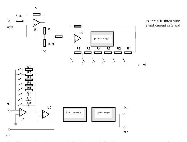
Hi and Lo are calibrator's output terminals. The stage including U1 operating amplifier converts voltage to current. U2 is a separation amplifier. R1 to R5 and C1 to C3 are range impedance. DA converter has 0 to +1 and 0 to +1 conversion ration and allows the simulation of resistance and capacitance values different from the range impedances. The output stage increases the permitted current load of the output.
