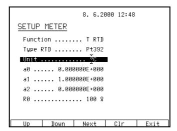
To reset the unit of measurement to original setting, press CLR display button. Original settings are listed below:
