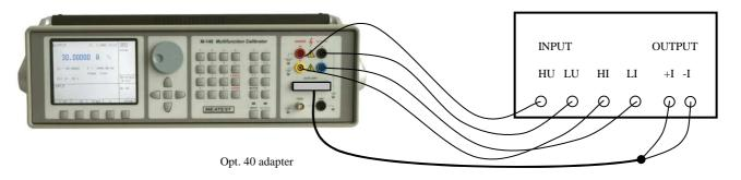
Function setup: Calibrator P function (voltage, current, power factor, frequency)
