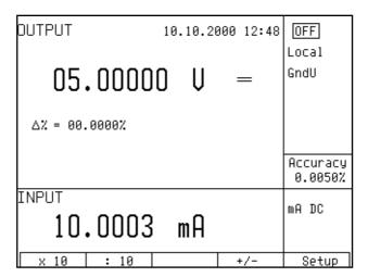
The multimeter does not display uncertainty of measuring. If the input range is exceeded, OVERFLOW message is displayed.
